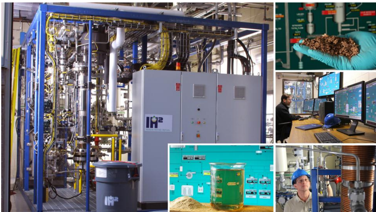
Figure 3: GTI's 50 kg/day IH 2 pilot plant.
