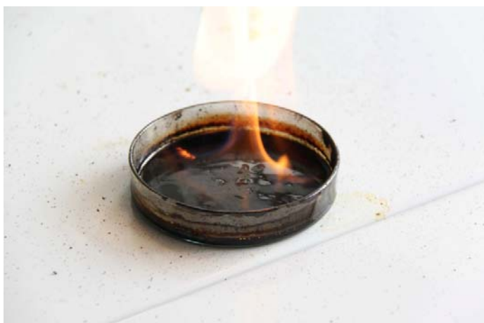
Figure 1: Pool fire combustion test of pyrolysis oil (KIT, bioliq).
