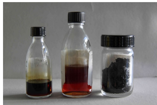
Figure 2: Distillation curve of pyrolysis oil (Chemviron, particle free); right picture shows solid foamy residue (right), first 50% distillate (middle), last 17% distillate (left).
