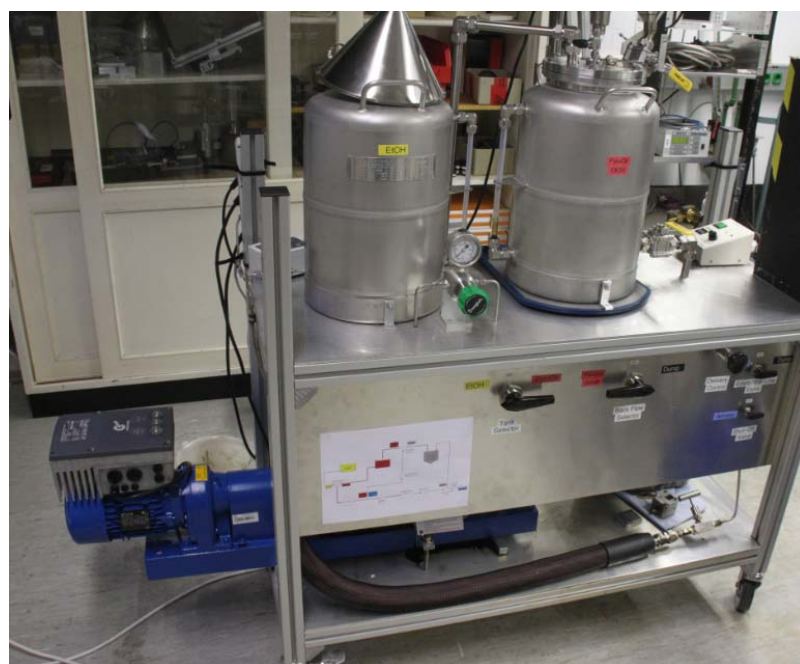
Figure 5: Set up for fluid delivery to the spray nozzle. The pyrolysis oil reservoir is equipped with a stirrer to prevent phase separation, the ethanol reservoir is mainly used to rinse the lines after tests are finished.
