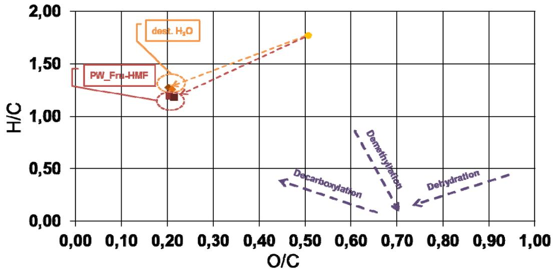
Figure 5: Results of hydrothermal carbonization shown in a Van-Krevelen-Diagramm.
