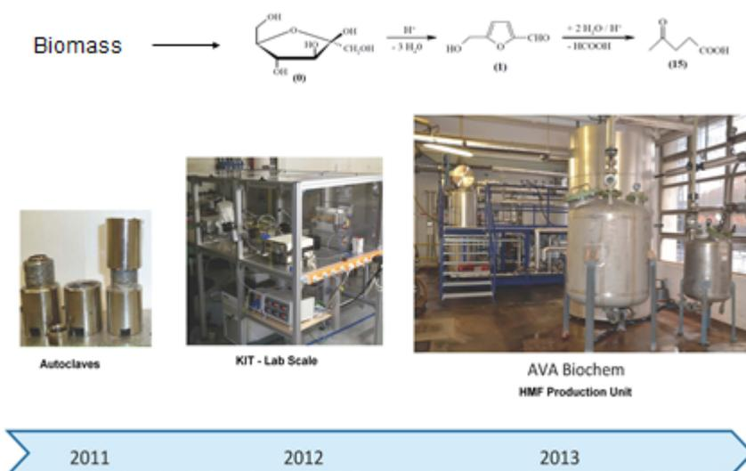
Figure 3: Illustration of the process development and scale-up of the HMF production process.
