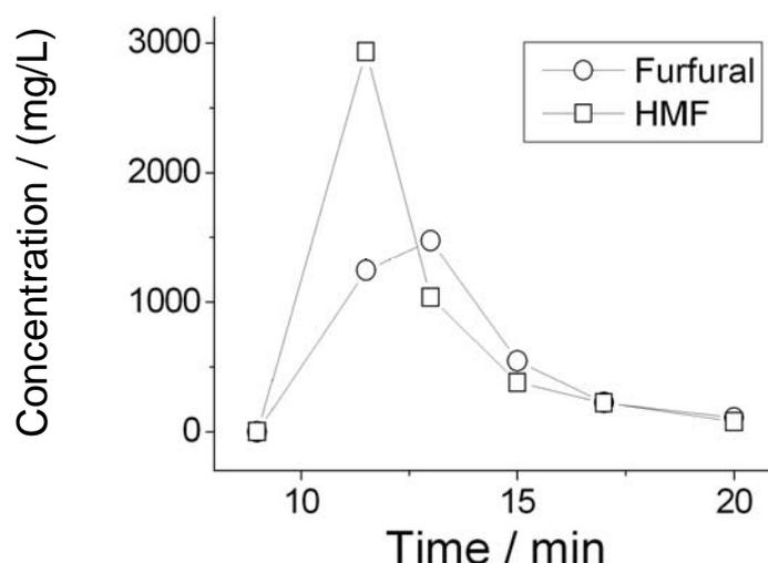
**Figure 1: Concentration of HMF and furfural from wood, extracted with hot water in a semi-batch reactor (200 °C, 3 mL/min water flow rate).**
