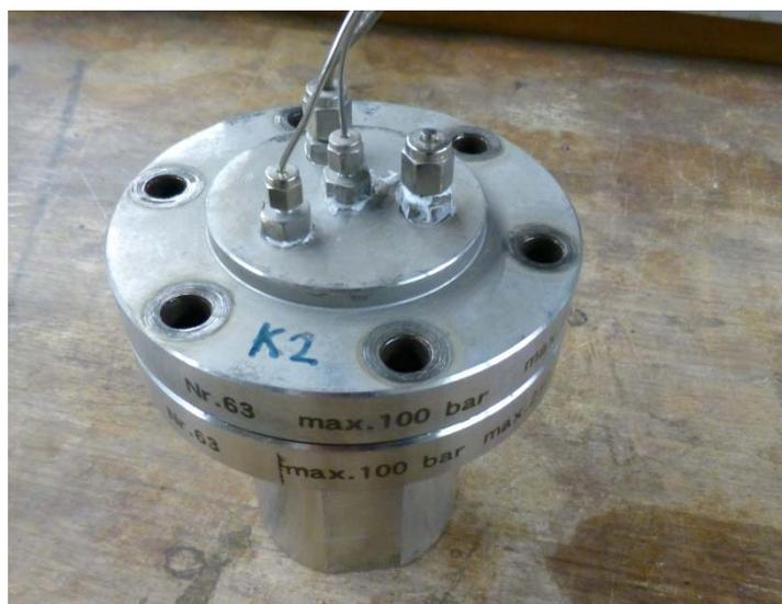
Figure 4: Autoclave in which the experiments were conducted (250 ml, stain-less steel).
