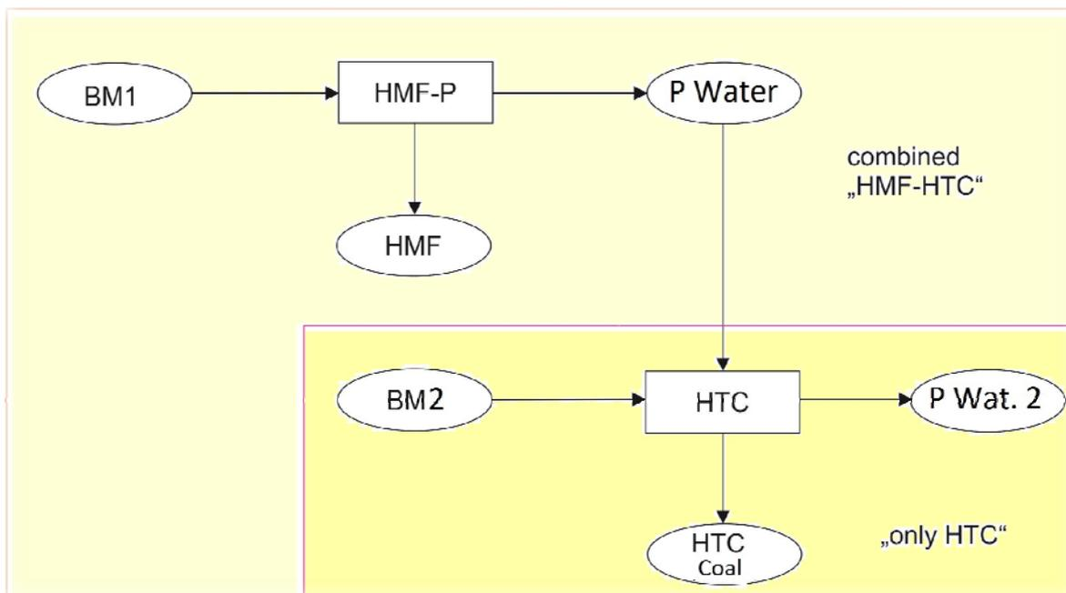
Figure 6: Coupling of HMF-production with HTC
