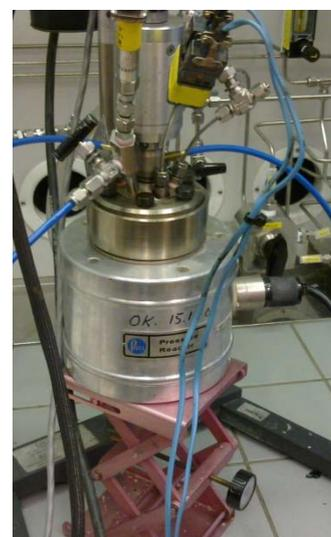
Prior to each experiment, the reactor is filled with about 50 grams of CPL, pressurized and left for 10-15 hours to ensure that the reactor is gas tight.
